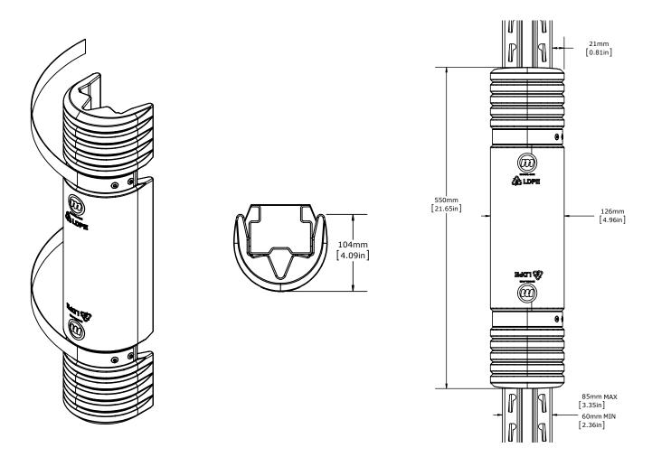
Rack Mounted Guard Kit Materials: Polyethylene body, hook & loop straps
